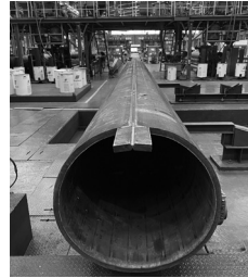
| STS-Clad 34"×34.1t×9M Tack welding 전 | | STS-Clad 34"×34.1t×9M Tack welding 후 |
